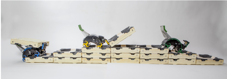
Harvard TERMES robots, based on termites
